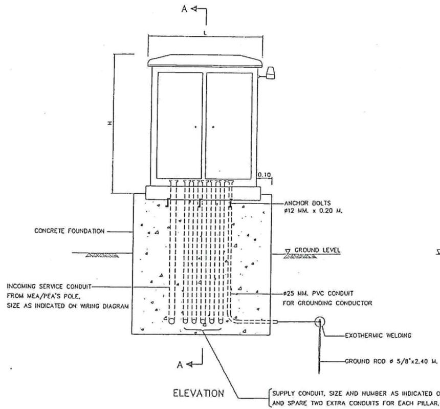
SUPPLY PILLAR ON CONCRETE FOUNDATION
