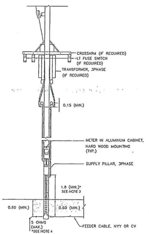
TYPE 3,4: FOR SUPPLY PILLAR NOT INSTALLED ON METERING POLE
