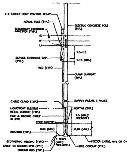
TYPE 1: FOR MEA'S OVERHEAD LINE, 1PH 2WIRE, NOT IN THE AREA OF UNDERGROUND CABLE PROJECT
