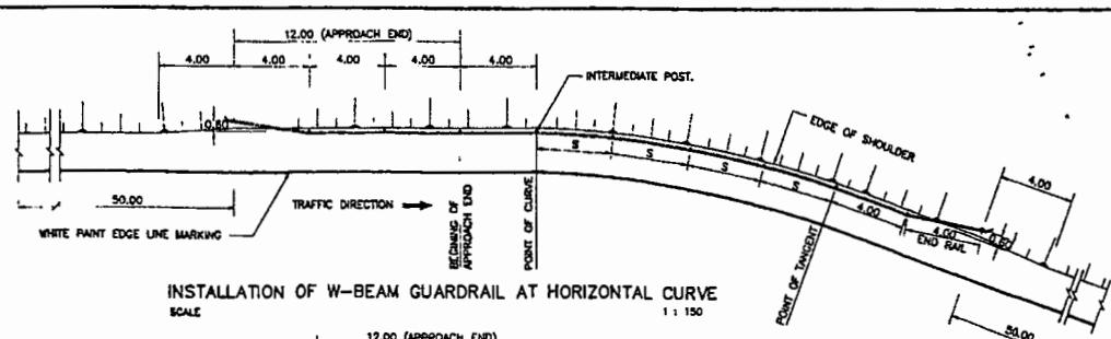
**INSTALLATION OF W-BEAM GUARDRAIL AT HORIZONTAL CURVE**
