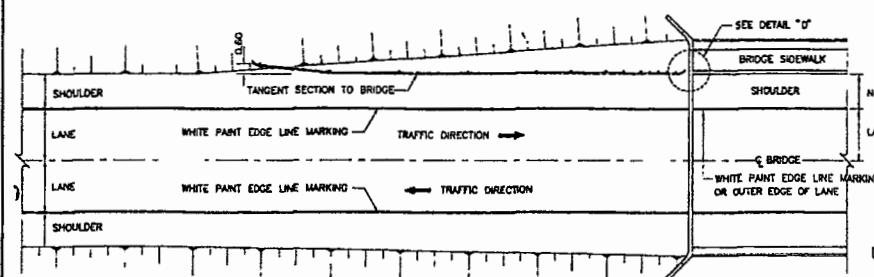
**INSTALLATION OF W-BEAM GUARDRAIL AT BRIDGE APPROACH WITH BRIDGE SIDEWALK
