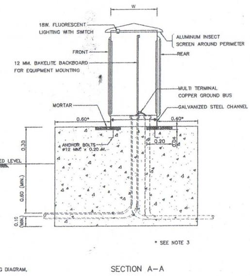
SUPPLY PILLAR ON CONCRETE FOUNDATION
