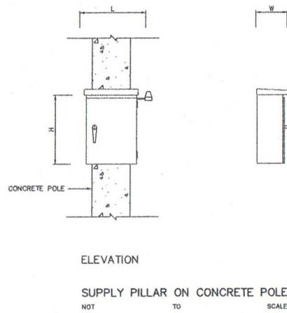
SUPPLY PILLAR ON CONCRETE POLE
