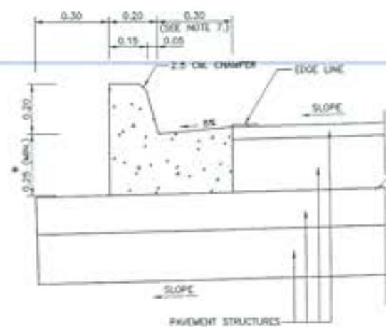
CONCRETE CURB AND GUTTER NOT TO SCALE
