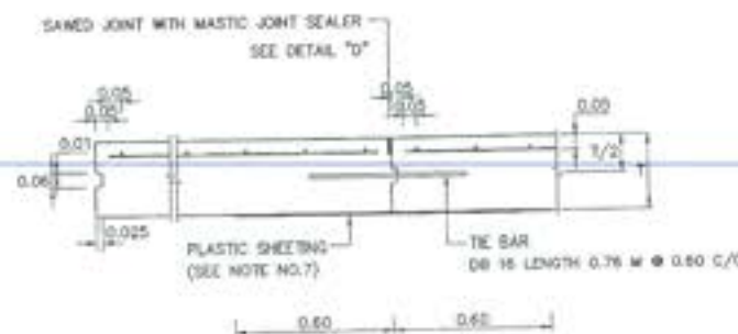
DETAIL OF LONGITUDINAL JOINT
